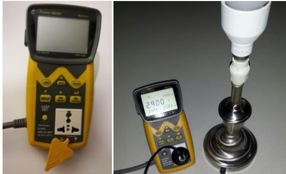
Figure 2: Power meter Wattman HPM 100A used for the measurements (Source: G. Dangl (left), S. Beletich (right)).
