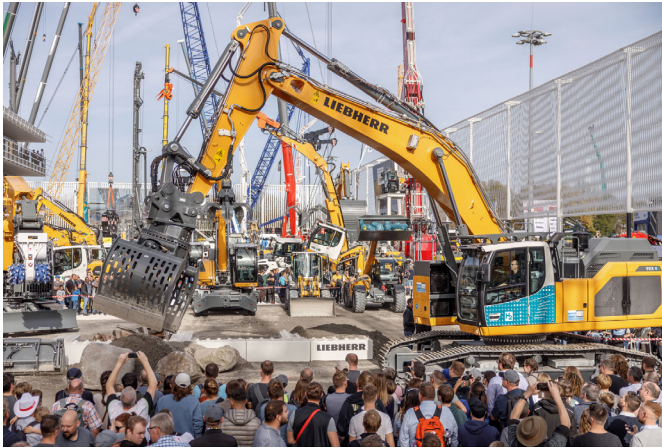
Figure 2: Presentation of crawler excavator demonstrator R 9XXH with hydrogen engine at Bauma in October 2022. © Liebherr-Werk Bischofshofen GmbH
