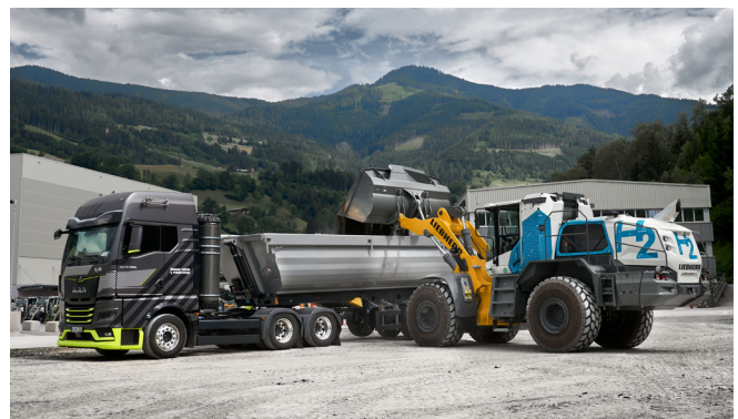
Figure 1: Hydrogen wheel loader prototype L 566H with MAN hydrogen truck, both vehicles powered by hydrogen engines. © Liebherr-Werk Bischofshofen GmbH
