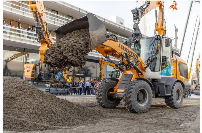
Figure 3: Presentation of wheel loader demonstrator L 507 Fuel Cell with hydrogen fuel cell at Bauma in October 2022. © Liebherr-Werk Bischofshofen GmbH
