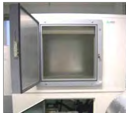
▲ Figure 4. A 5 kg test stand for thermochemical storage at EDF.
