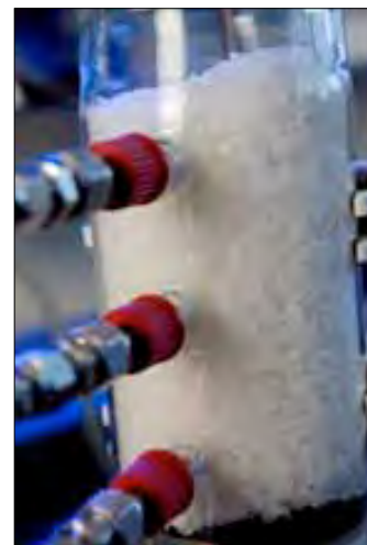
▲ Figure 2. Small experimental reactors to determine the hydration/dehydration characteristics of salt hydrate composites at ECN.
