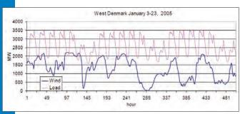
Figure 1. Wind power production (2,400 MW wind power) and load in Western Denmark.
