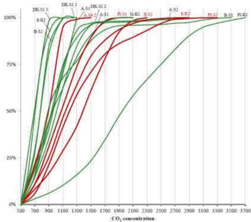
Figure 16 Cumulative distribution chart showing % of time with carbon dioxide (CO<sub>2</sub>) concentrations below or above certain level; green lines show CO<sub>2</sub> concentrations in frontrunners and red in the reference conventional buildings. There is a systematic difference in the measured conditions between the two different types of buildings, CO<sub>2</sub> concentrations being generally lower in frontrunner buildings
