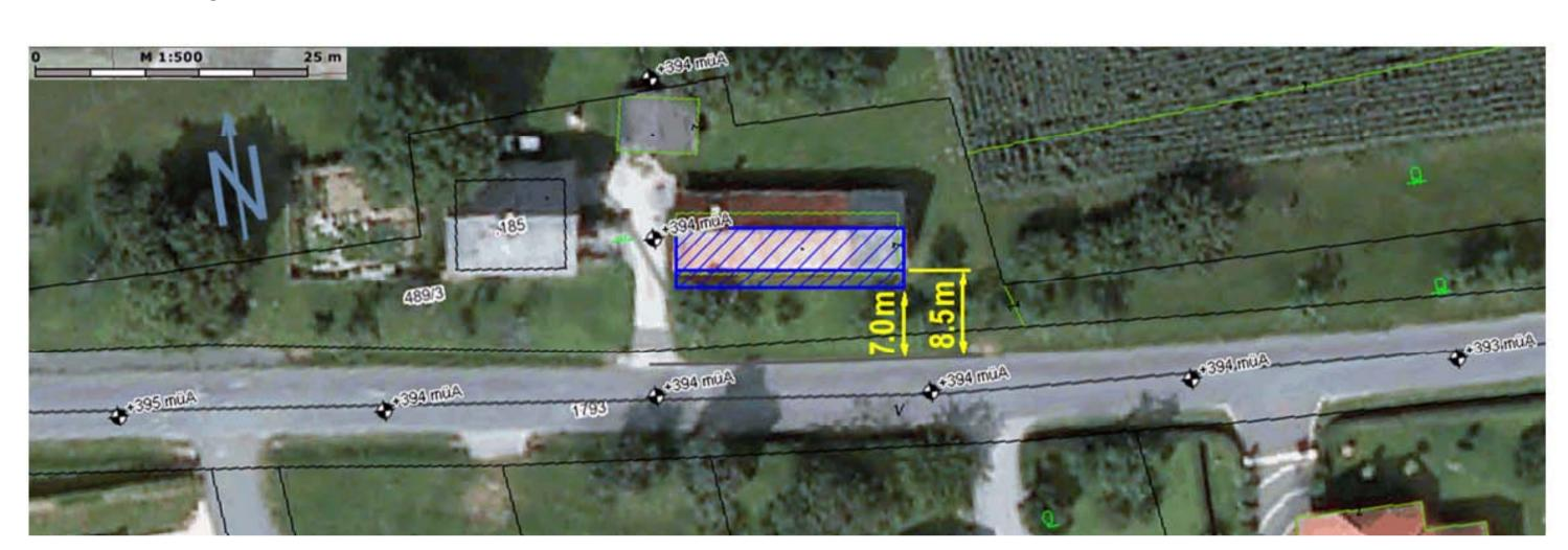
The reflection of the roof integrated PV setup is assumed critical, if it illuminates a strip by the height of a lorry over the center line of the road. City officials wanted to have an estimate on when and how intense the glaring affects the traffic.
