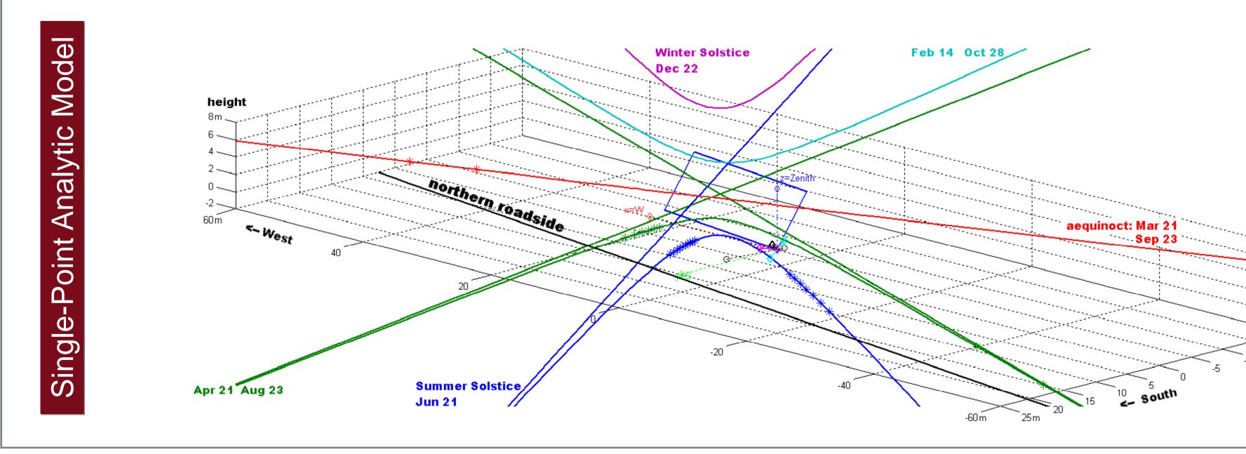
By simplifying the whole roof as a small source when viewed from the street, the reflected light path can be analytically calculated and intersected with the ground surface and the plane above road's center line.
