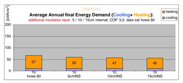
Graph 91: Final Energy Demand due to additional layers of internal insulation in ONB
