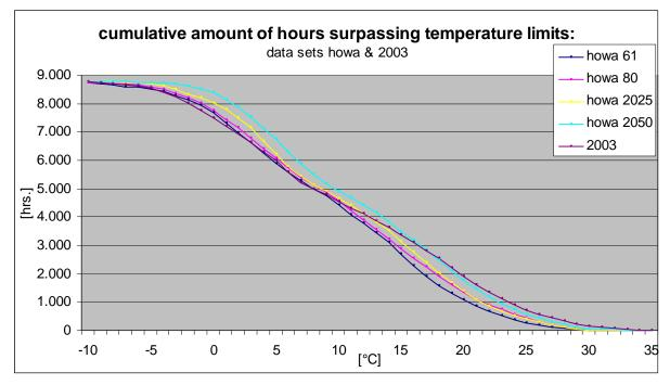
Graph 12: Amount of hours surpassing continuous temperature limits for different temporal resolution of howa
