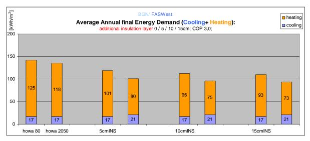
Graph 92: Final Energy Demand due to additional layers of internal insulation in BGN/ FAS
