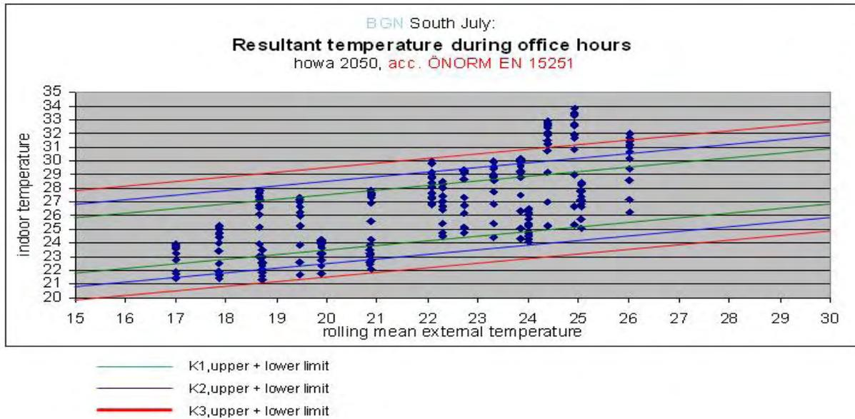
Graph 78: Resultant temperature in BGN under data set „howa 2050“ acc. to EN 15251 **Fehler!**
