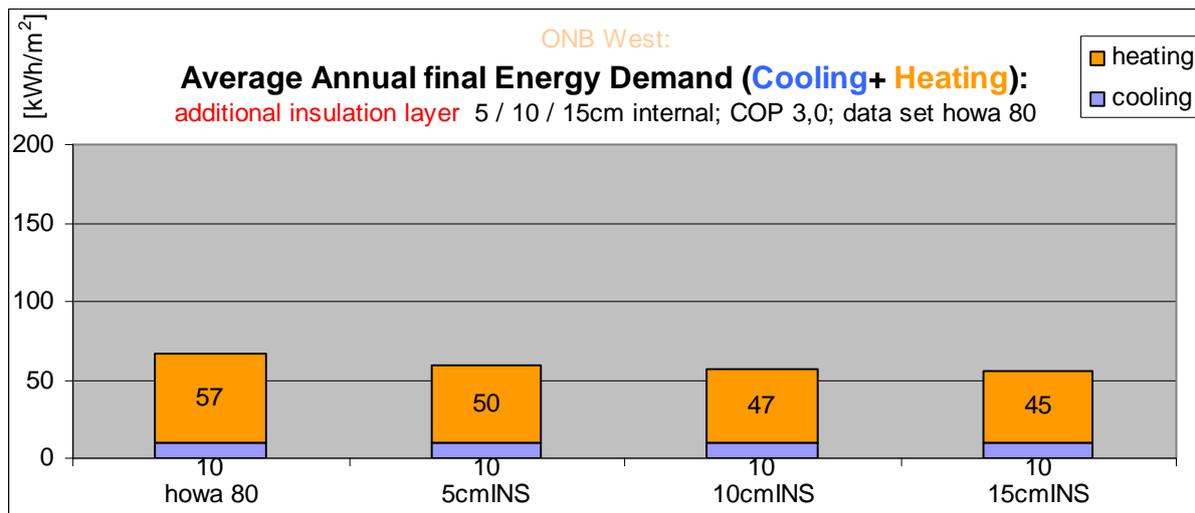
Graph 91: Final Energy Demand due to additional layers of internal insulation in ONB
