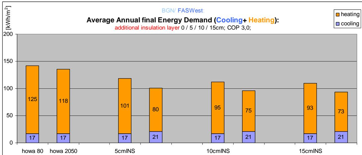
Graph 92: Final Energy Demand due to additional layers of internal insulation in BGN/ FAS
