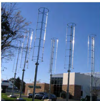
Wind school. Placing vertically aligned turbines closer together gives more wattage for the buck. Credit: Marsh Power. CLOSE X
