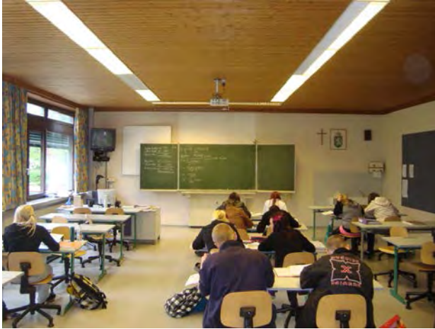
Figure 13: Dark ceiling and shaded disregarded windows lower the incidence of daylight
