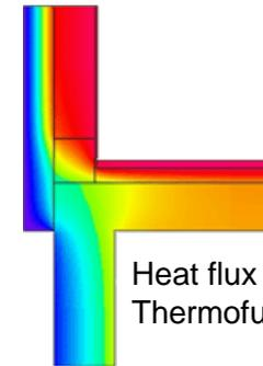
Heat flux with Thermofuss plus
