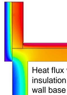
Heat flux without insulation of the wall base
