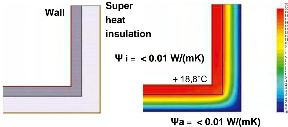
Geometric thermal bridges are not longer relevant !!!
