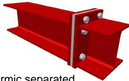
Thermic separated end plate joints
