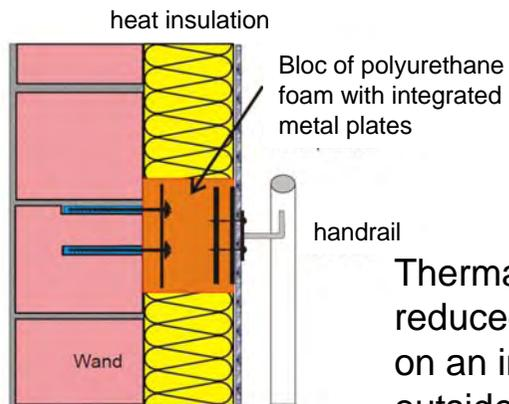
Thermal bridge reduced fixing on an insulated outside wall
