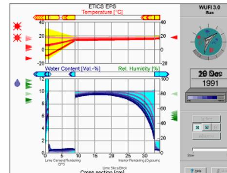
The time steps for the climate data and the calculation may be selected at the user's discretion; for most cases hourly values are appropriate. It also writes a film file during the calculation which contains all the computed profiles and which - displayed as a 'film' - conveys a dynamical impression of the thermal and hygro processes in the component.
