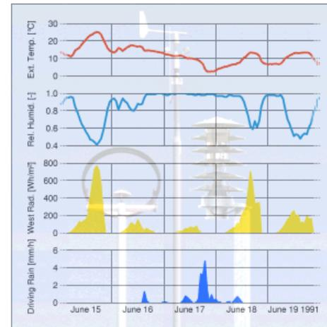
The boundary conditions acting on the building component are the temperature and relative humidity of the interior and exterior air and the rain and radiation loads, both depending on inclination and orientation of the building component. These data can be derived from a database. ASHRAE provided the raw data for the development of a moisture design year for 50 cities.
