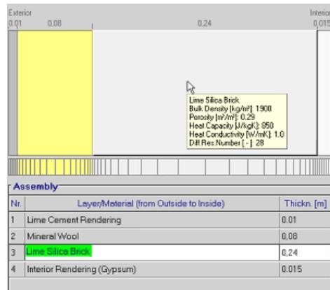
The individual layers of the component and their respective thickness are entered into a table.
