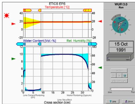
After entry of a few remaining data like surface transfer coefficients, initial conditions etc., the calculation can be started. It then computes the temporal evolution of the temperature and the moisture field in the component.
