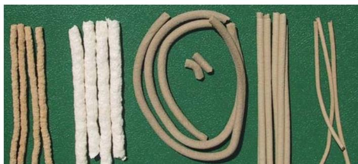
bright colour and a smooth surface. They were fine pored and in addition more rigid than the original mixture. Different recipes showing good expansion and relatively high strength were however sometimes too brittle.
