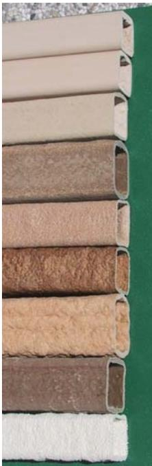
As preliminary test to the profile extrusion foamed strands were extruded with a slot die. At low number of revolutions the expansion was better, but the surface was irregular; at higher number of revolutions a smoother surface but less expansion were obtained; partly the feeding capacity of the powdery substances was low; after a screw exchange (screw with higher shear action) a high expansion was observed, the surface remained however irregular.
