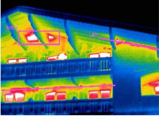
A thermal image of a roof structure. The roof is highlighted in red and yellow, indicating heat loss. The surrounding walls and ceiling are shown in blue and green. A pink box highlights a specific area on the roof, and a pink line points to a connection point on the wall.                  |
