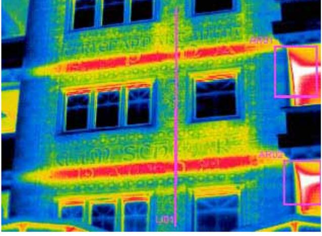
A thermal image of a building facade. The walls and ceiling are highlighted in red and yellow, indicating heat loss. The surrounding area is shown in blue and green. A pink box highlights a specific area on the wall, and a pink line points to a connection point on the ceiling.             |
