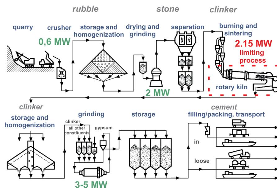
Fig. 2: Basic process chain in the cement industry (source: based on VDZ)
