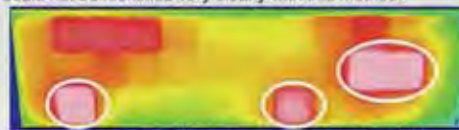
Fig.2: Illuminated IR-Thermography, sc-Si-module
