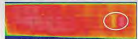
Fig.3: Dark IR-Thermography, sc-Si-module
