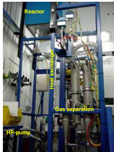
Reactor & gas separation
