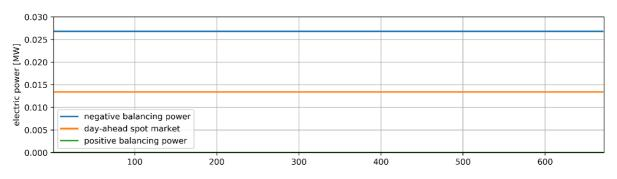
Figure 6: optimal bidding strategy for the heat pump (1 week). Use case: B3.1-SW.
