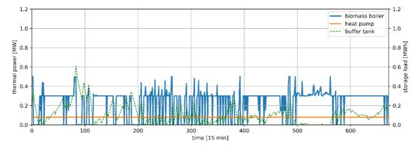
Figure 5: optimal operation of the biomass boiler, heat plant and storage for 1 week (15-minutes basis time step). Use case: B3.1-SW.
