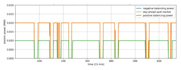
Figure 4: "high" bidding strategy for the heat pump (1 week). Use case: B3.1-SW.
