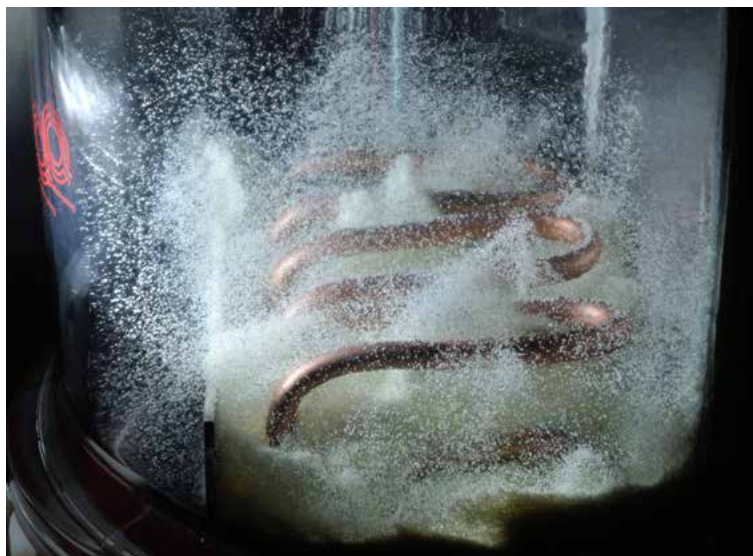
Fluidised bed layer of the absorber, Photo: TU Wien/Julius Pirkbauer
