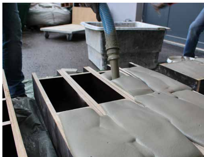
The first experiments using novel formulas for concrete that result in better heating insulation have already been conducted, Photo: Smart Minerals GmbH
