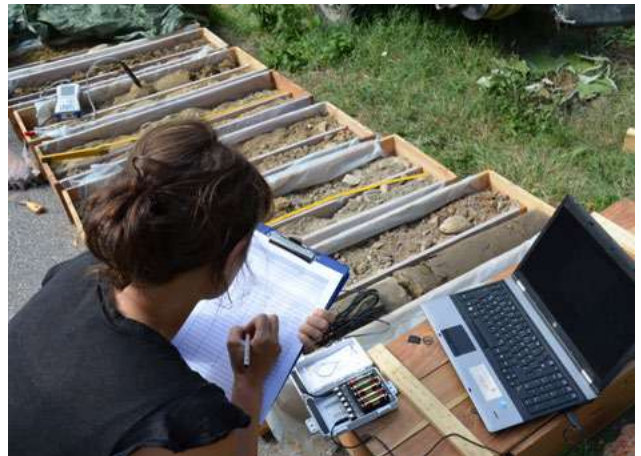
Thermal conductivity measurements on the drilling core, photo: Heat Harvest consortium
