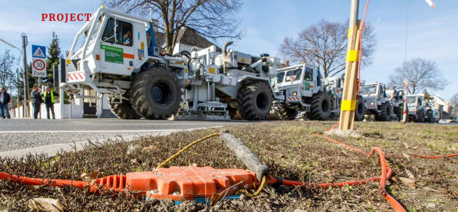
"Pulse vehicles" for carrying out 2D seismic measurements in the regions of Vienna and Groß-Enzersdorf, photo: Wien Energie/Christian Hofer
