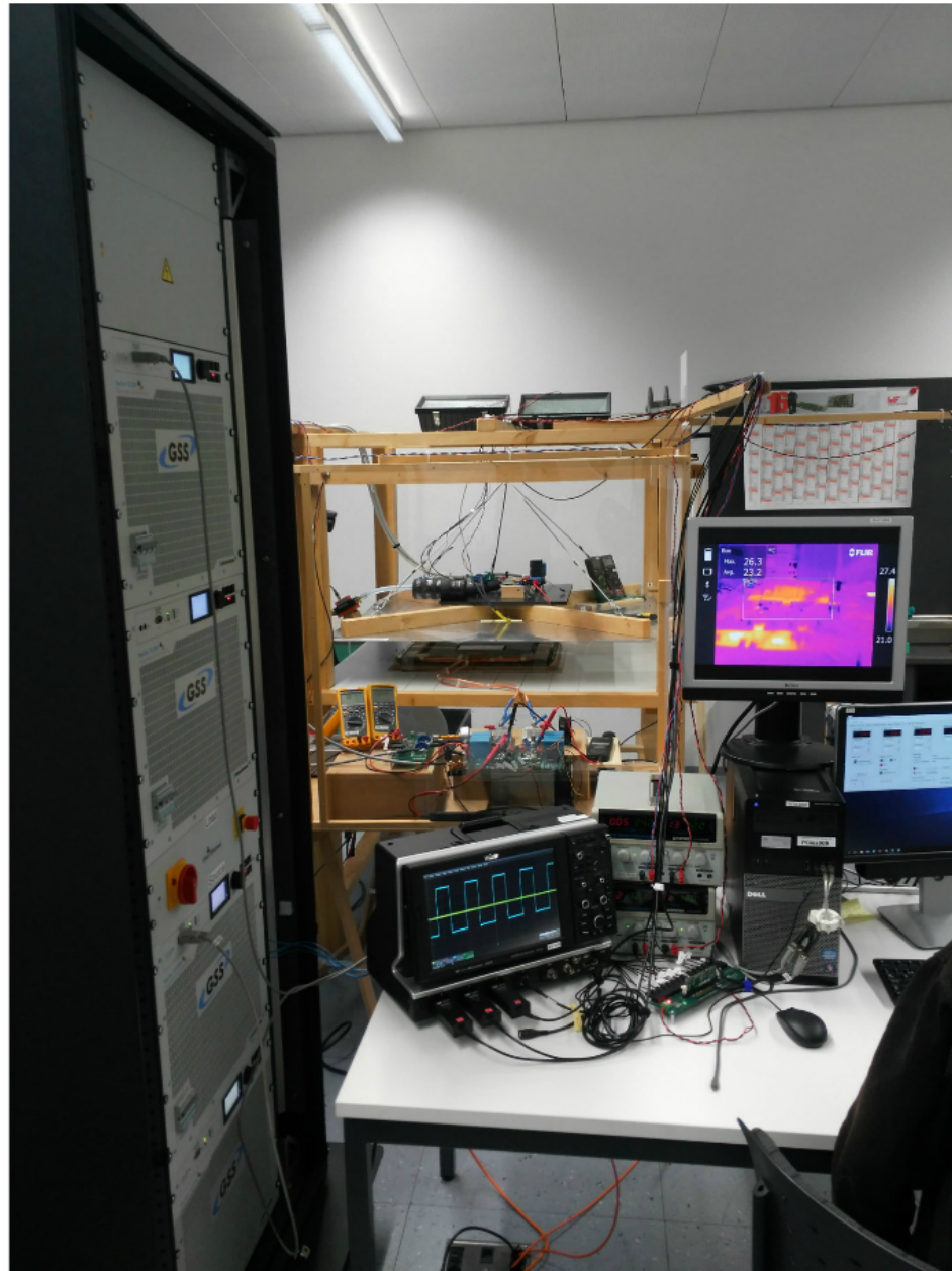
Early Testsetup of 22 kW System Efficiency up to 96 %
