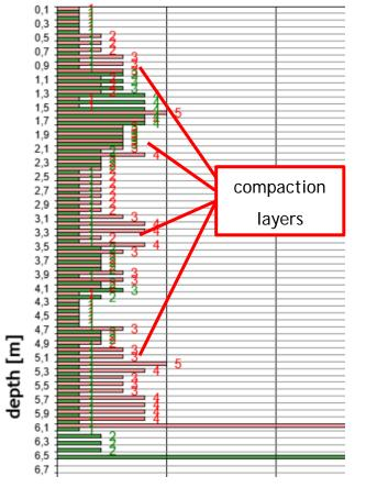
ram penetrometer tests
