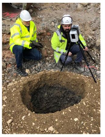
borehole laser scanning
