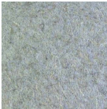
Fibrimat F300 / F450 300 g/m 2 / 450 g/m 2 (EcoTechnilin, France)
