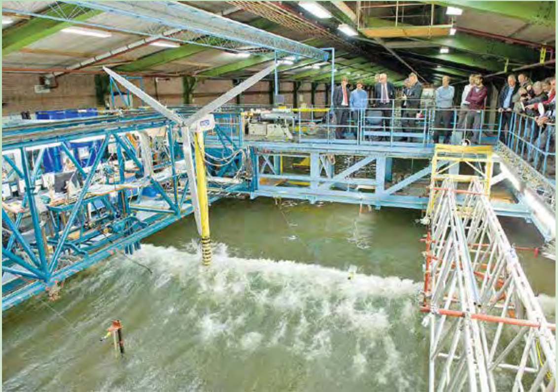
Figure 3. Marin Splash: A test of the impact of breaking waves on support structures in Marin's shallow water basin
