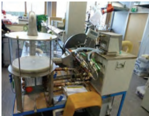
Figure 8: Left: Bulk type open sorption prototype reactor of ECN. Right: system design.
