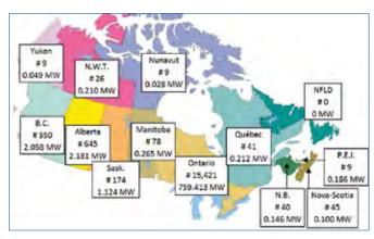
Fig. 2 - Map showing the Canadian provinces, the capacity (megawatt) and the number of utility interconnected PV Systems in 2012.
