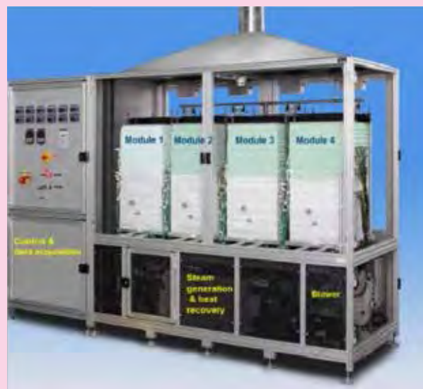
Figure 11: 20kW SOFC system based on four 5kW stacks by Forschungszentrum Jülich
