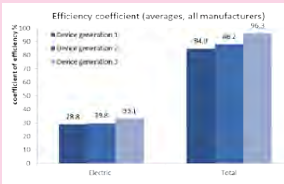
Figure 16: Efficiency coefficient (CE test standard) for CHP FC generation 1, 2 and 3 under the Callux project
