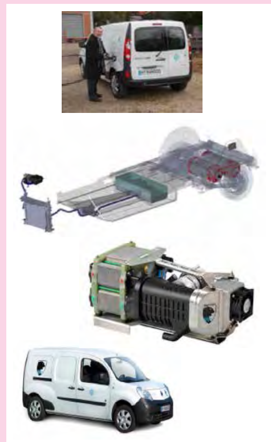
Figure 22: The HyKangoo from SymbioFCCell and Renault, an electric van with a hydrogen fuel cell range extender
