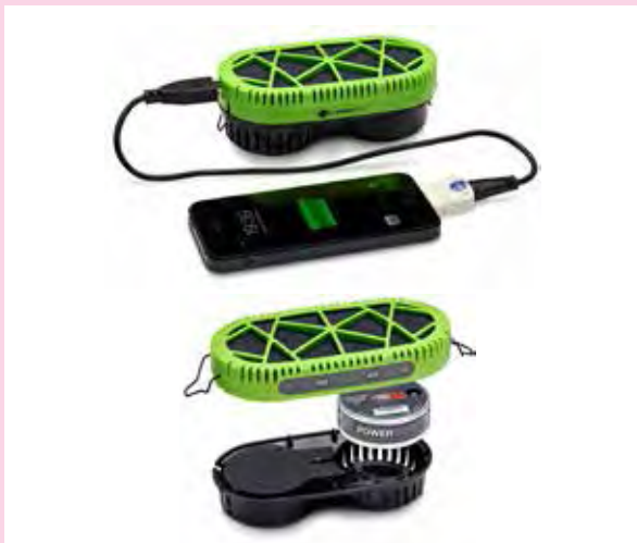
Figure 26: myFC portable charger for electronic gadgets, and the power puck cartridges (Source myFC)
