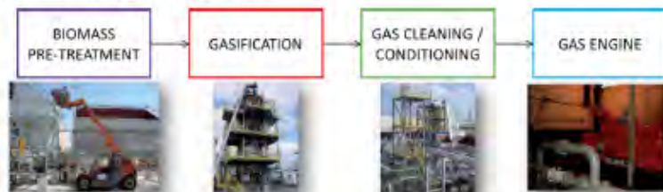
Configuration of a small-scale gasification plant
