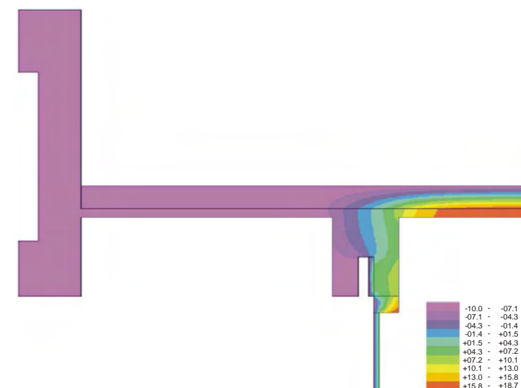
Picture 2-1: Typical thermal bridge of a projecting roof with an concrete attic (Source: Arch. Erwin Kaltenegger)
