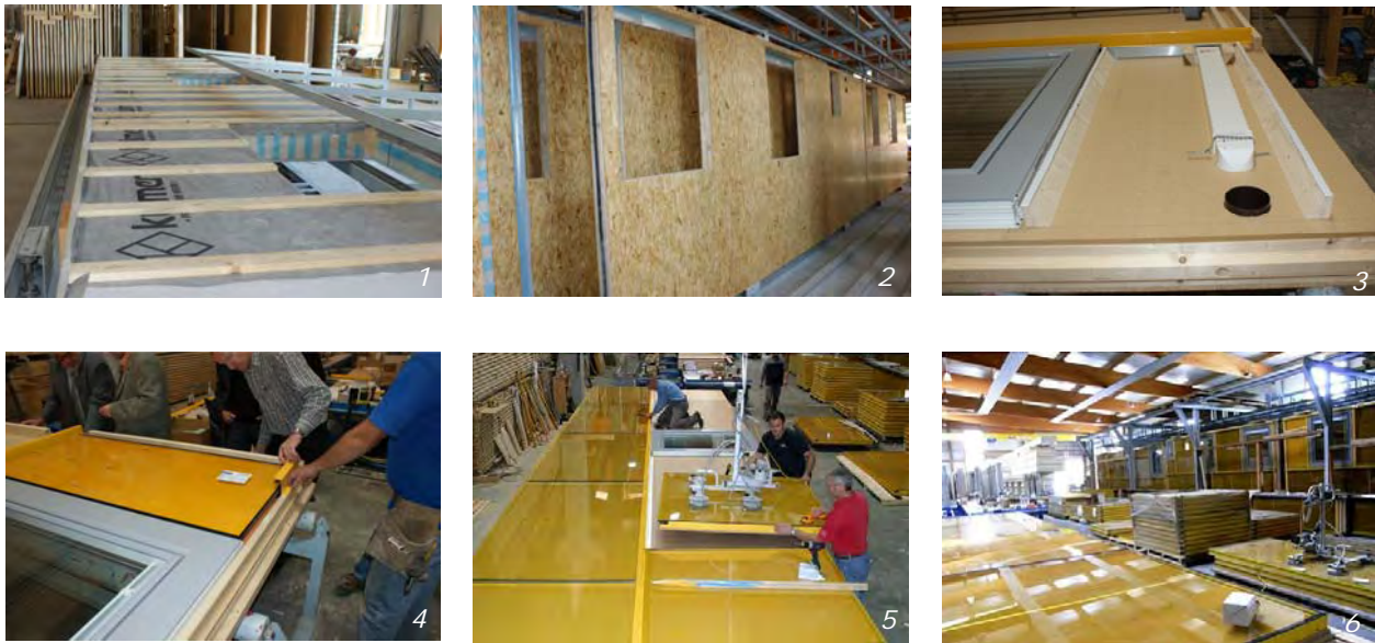
Figure 16: Sequence of prefabrication procedure in the fabrication hall (Source pictures 5-6: Gap-Solution GmbH)
