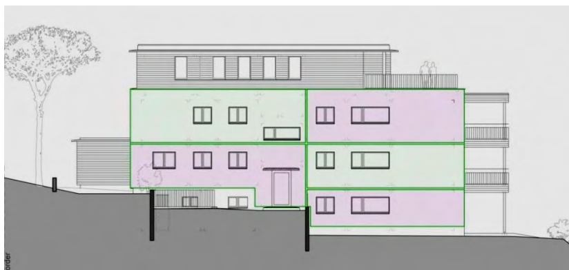
Figure 25-26: Module prefabrication for north-west façade (left) and south-west façade (right)
