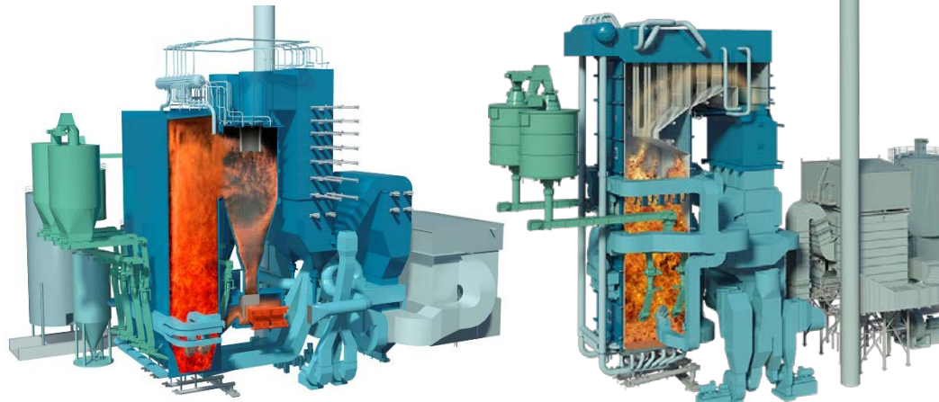
CFB Boiler Plant
