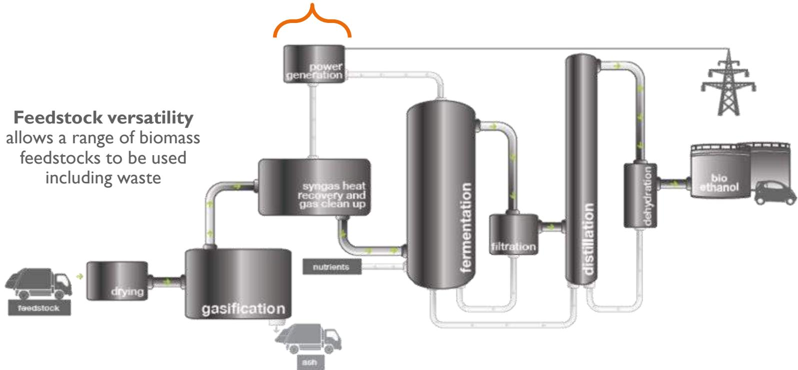
**Feedstock versatility** allows a range of biomass feedstocks to be used including waste
