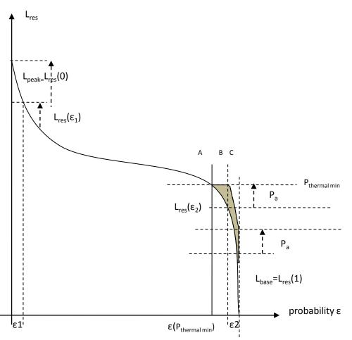
The energy curtailment is the area below the Thermal Minimum Load and above the Customer Load
