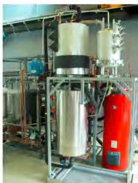
EMPA's liquid sorption reactor with two separate stages.
