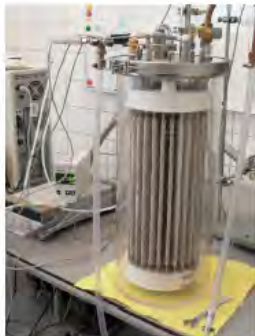
TNO's prototype sorption reactor with solid sorption material attached to the fins of the heat exchanger.
