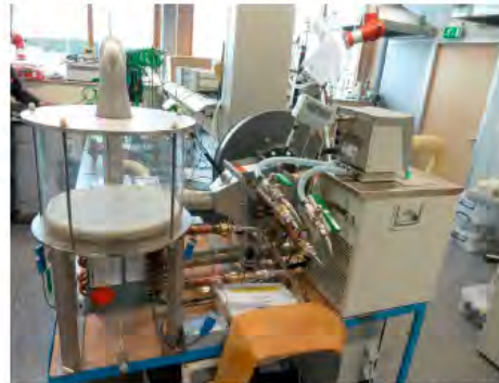
ECN's bulk type open sorption prototype reactor.
