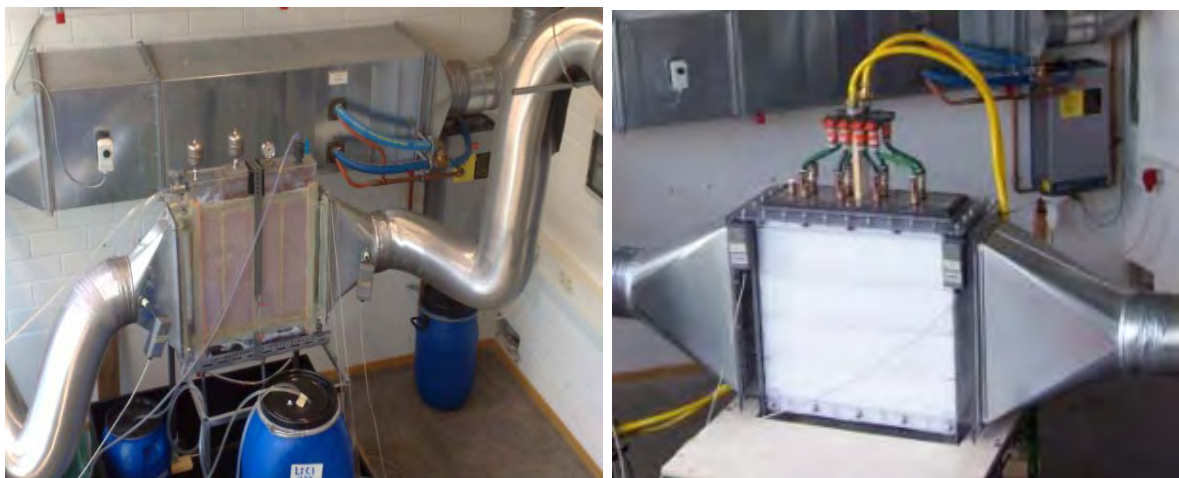
Figure 27: Non-adiabatic liquid desiccant absorber/regenerator (left) and adiabatic liquid desiccant absorber (right) made-out of polycarbonate in the pilot plant stage in the laboratories of Kassel University. Jaradat et al [120].
