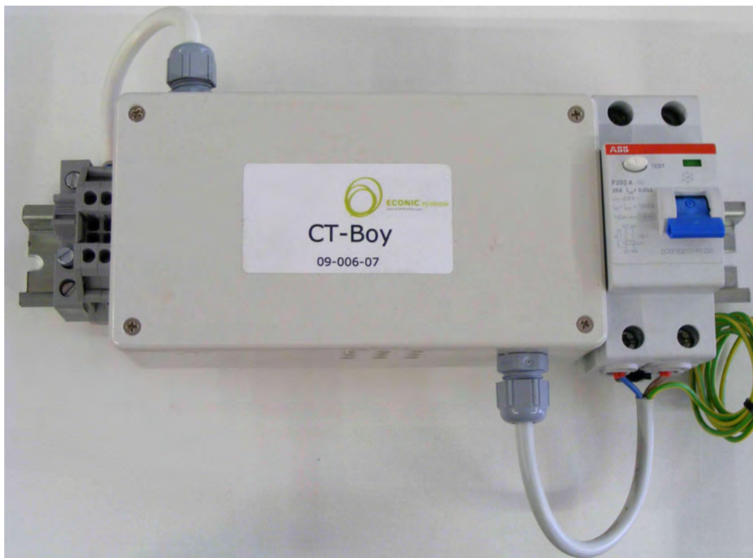
Figure 5-8: Test device for silver/copper ions production (courtesy of ECONICsystems)
