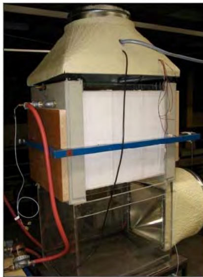
Figure 26: Non-adiabatic liquid desiccant absorber/regenerator made-out of polypropylene, University of South Australia, Krause [116]
