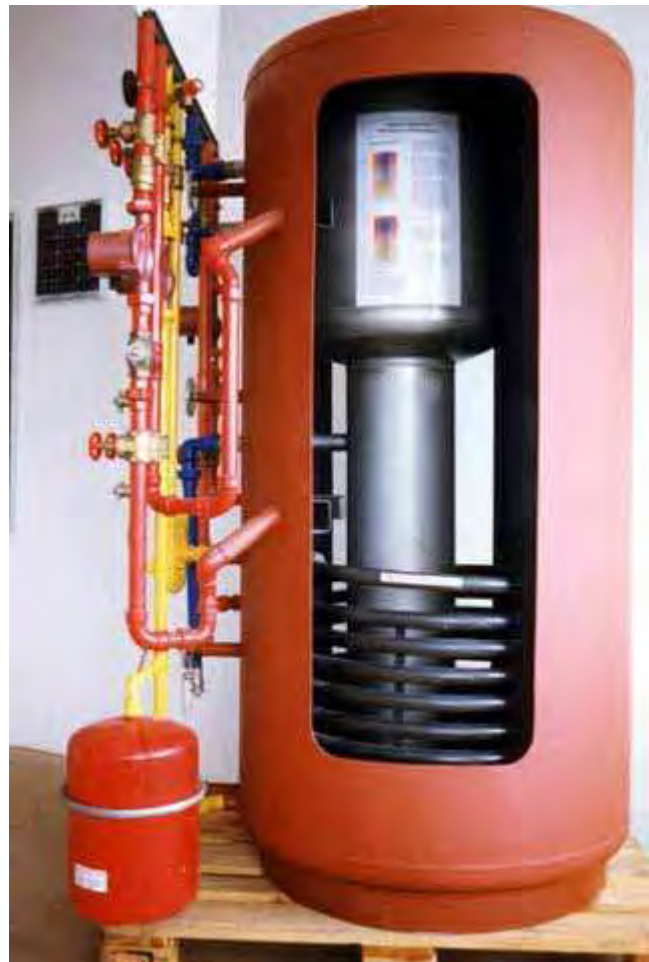
Fig. 3: Tank-in-tank system (Jenni, CH)
