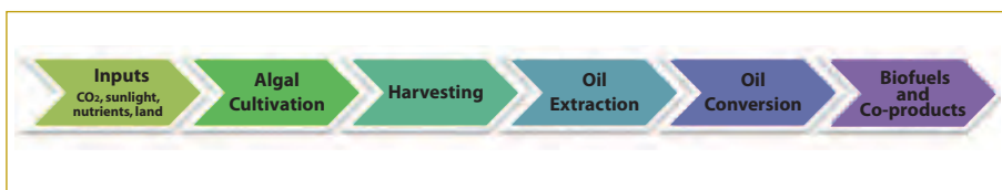
Figure 1. Simplified schematic diagram of major steps involved in producing algal-derived liquid biofuels.
