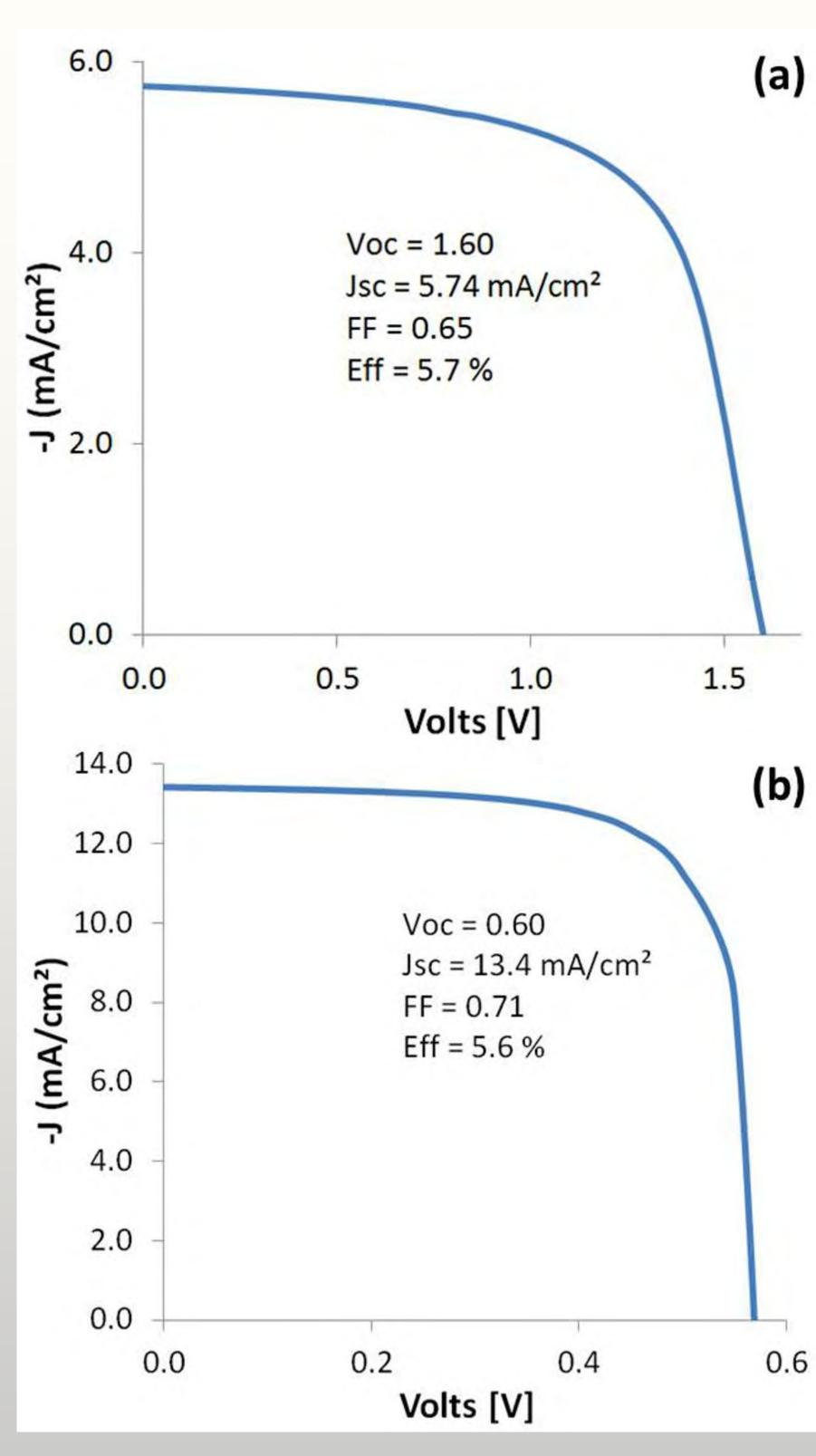
(a) Simulated AM1.5G J-V plot of an a-Si p-i-n(Eg=1.8eV)/p-i-n(Eg=1.6eV) device; (b) sim. AM1.5G J-V plot of a-Si p-i-n(Eg=1.4eV) device.
