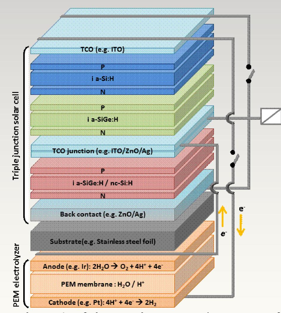
Schematic of the novel concept: The current of the upper dual junction enables the water splitting reaction in the PEM electrolyser. Contacts, possible wiring, currents, and water dissociation reaction are shown schematically.
