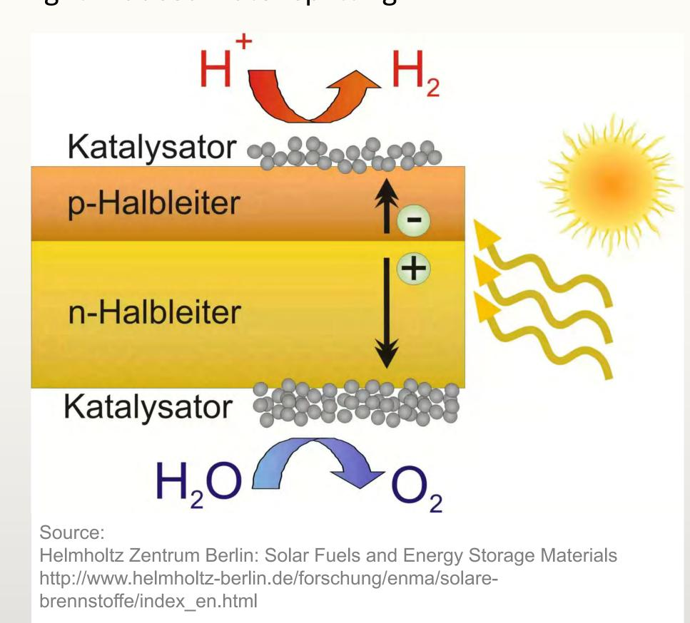
The solar splitting of water to hydrogen and oxygen driven by photon energy is schematically shown above.
