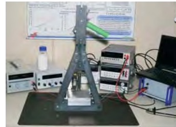
Left: Hot embossing set-up developed on TUW, right: one embossed sample (polycarbonate layer over the solar cell)
