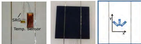
Left: Photograph of the sensor setup Middle: PV mini module Right: Schematic view of the 45° rosette
