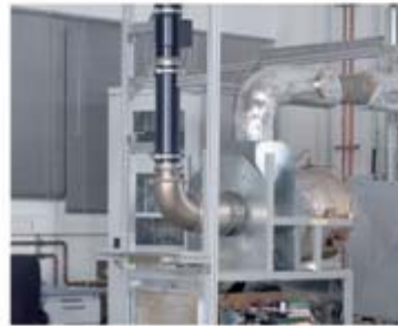
Hydrogen powered microturbine in a test rig
