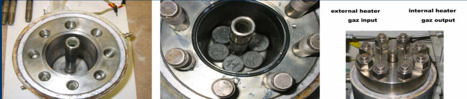
Experimental design, titanium made vessel, (opened, at left) , disposition of two material cores crown in the vessel, vessel closed in its running configuration (right)
