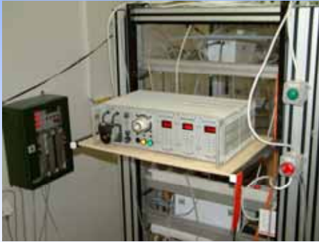
Gas analytic for raw gas & cleaned gas, Micro GC for MCFC gas analytics (not on the picture)
