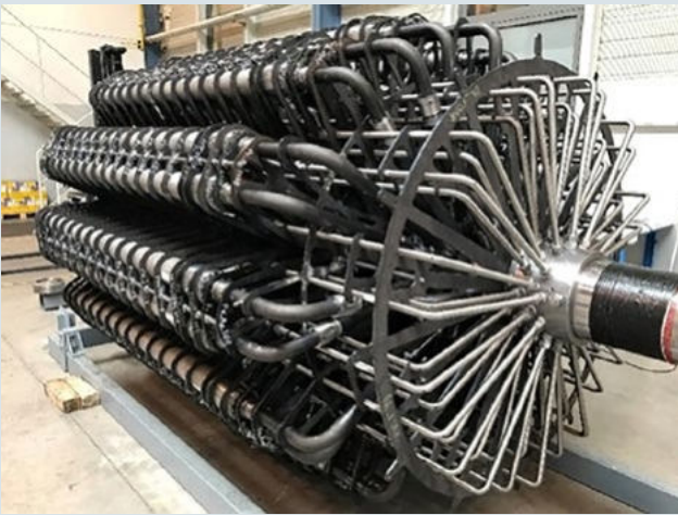
Rotation heat pump, photos: ecop
