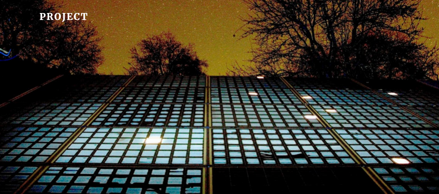
PV modules lit with ultraviolet light/ UV fluorescence (UVF) method for detecting effects of ageing, photo: AIT/B. Kubicek
