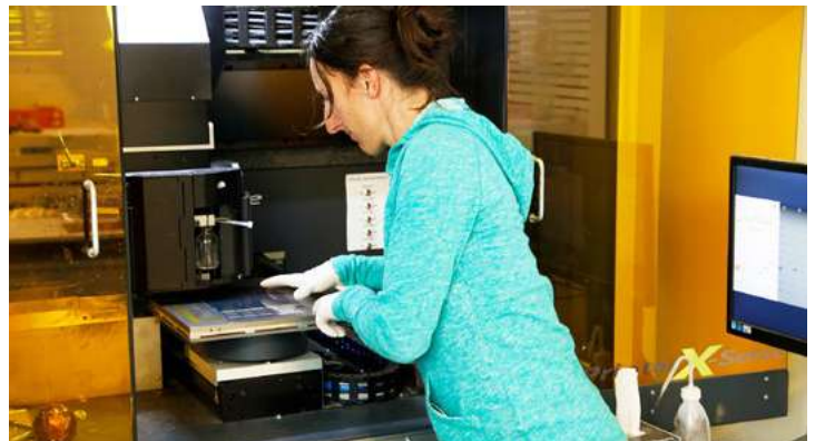
Serial interconnection of thin-film solar cells using inkjet material printing, photo: Sunplugged
