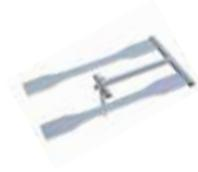
The formulation is process able in the conventional injection moulding process. Test bars are used for the mechanical characterisation.
