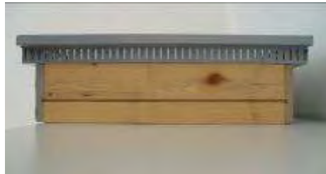
Picture 21: The prototype of the facade module. The timber frame and the ventilation slots can be seen.
