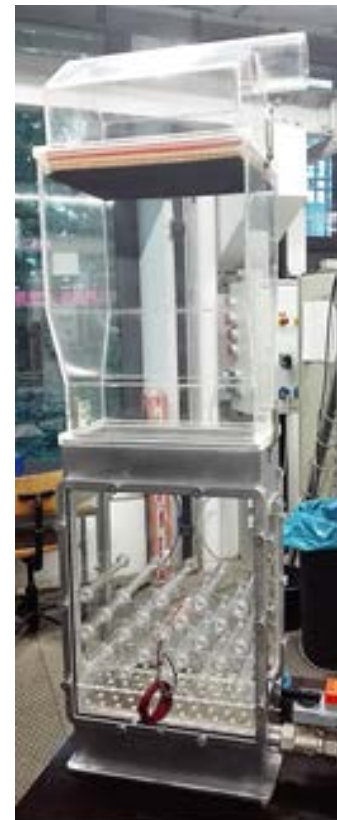
Abbildung 18 Bubbling fluidized bed heat exchange testing device in horizontal tube modification.
