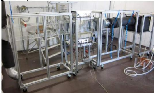
Figure 16: Test facility for experimental analysis of flue gas condensation @ AIT (Seichter et al., 2013)
