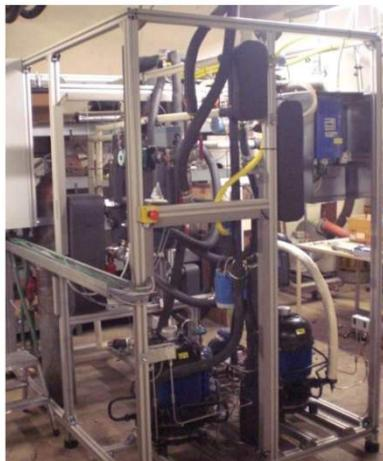
**Figure 12: Picture of the absorption-/compression heat pump prototype @ IWT (Hannl & Rieberer, 2014)**
