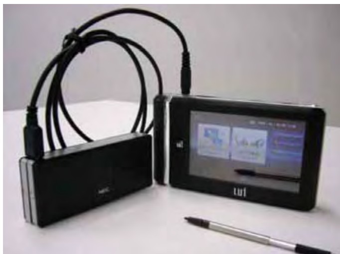
Figure 4.62 Prototype FC pack with a power output of 3 W (max. 5 W); external size: 110 mm x 45 mm x 20 mm (Source: NEC, Japan)
