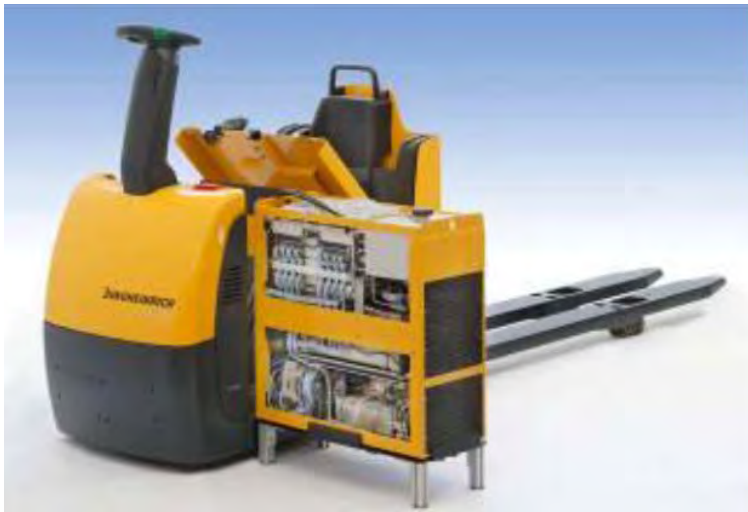
Figure 4.57 Warehouse truck with DMFC system; 7 kW peak; 0.8 kW average; fuel: pure methanol (Source: Forschungszentrum Jülich, Germany)
