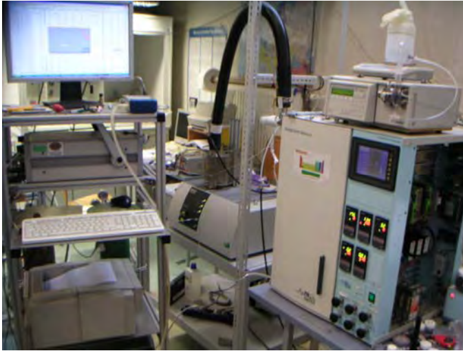
Figure 4.65 Experimental facility: Catalytic test bed (left), Micro-Gaschromatograph (right) and Mass Spectrometer (middle) (Source: Fuel Cell Lab TUG, Austria)
