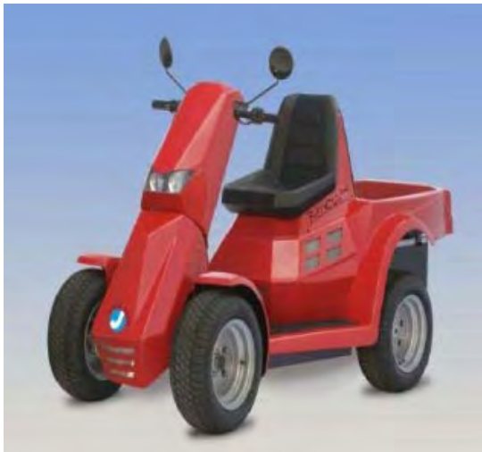
Figure 4.12 JuMOVE2 which showed stack degradation of 1,800 W to 600 W over 500 operating hours (Source: Forschungszentrum Jülich GmbH, Germany)
