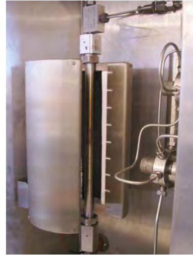
Figure 4.66 Hot-box with reactor heater and stainless steel reactor (Source: Fuel Cell Lab TUG, Austria)
