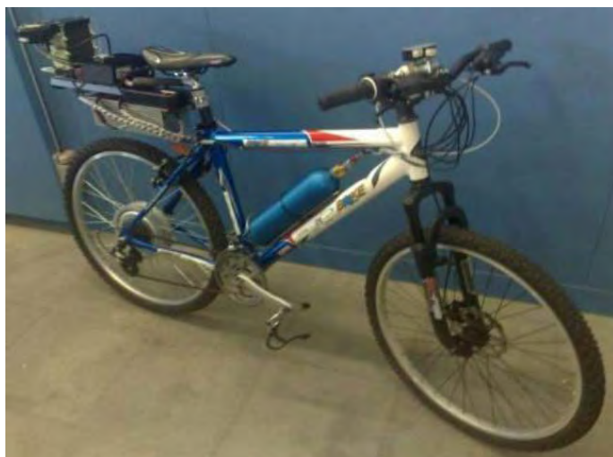
Figure 4.58 250 W PEFC bicycle; hydrogen storage pressure: 0.7 - 0.8 bar; PEFC with 22 cells (31 cm 2 active area) (Source: ITAE, Italy)
