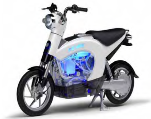
Figure 4.59 DMFC scooter with a system efficiency of more than 32% (Source: YAMAHA, Japan)
